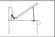
**To lower the top:** Hold the front edge of the cooktop and carefully push back on each support rod to release the notched support. Then gently lower the top into place. The support rods will slide into the range frame.
