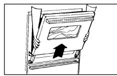
**CAUTION:** Hinge arms are spring mounted and will slam shut against the range if accidently hit. **Never place** hand or fingers between the hinges and the front oven frame. You could be injured if hinge snaps back.
